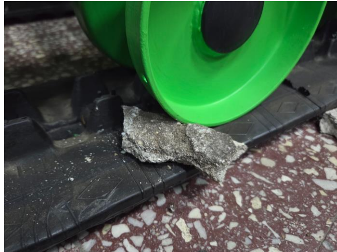
Fig. 3. Detail capture: interaction between the roller and a piece of concrete caught in the track
