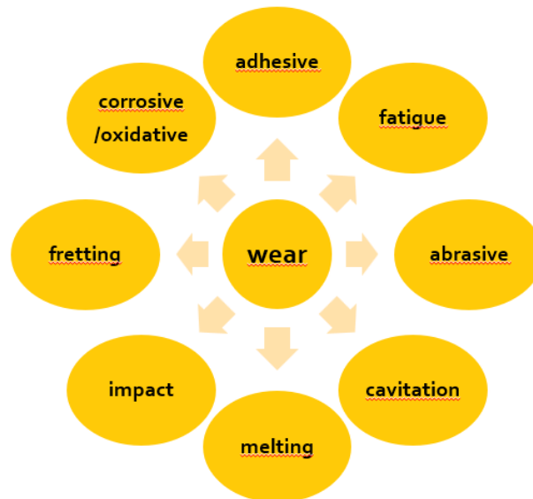
Fig. 2. Main types of wear in hydraulic systems
