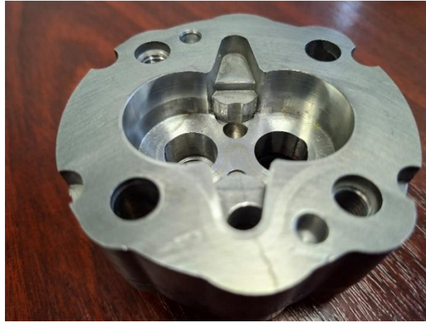
Fig. 4. Gear pump housing with wear evident in the suction and discharge area
