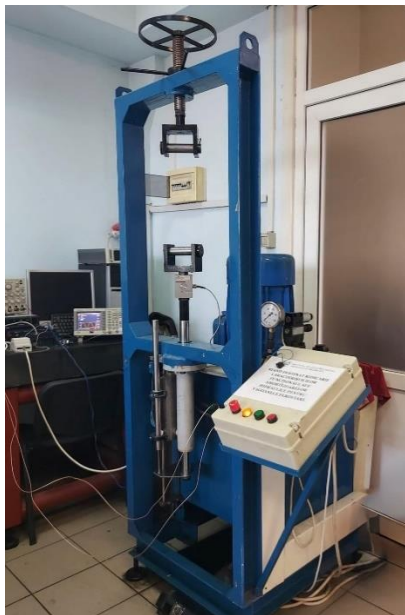
Fig. 1. Shock absorbers test stand with rigid pipes
